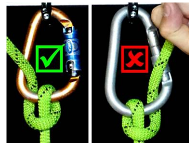
Fig 2. Correct orientation of the control line away from the carabiner gate (Left) and incorrect orientation (Right). Here the control line is not in the brake position (cf Figs 1, 3.) From https://www.ropelab.com.au/munter-hitch/
