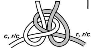
The unusual asymmetry of interlocked thumb knots in a (loose) Lineman's Bend
