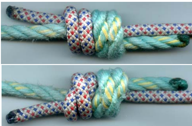
Fig. 8. Double overhand bend (grapevine, double English, or double fisherman’s knot, ABOK #1415) viewed from the front and rear. Stronger but more prone to jam than a Flemish bend (Fig. 7).
