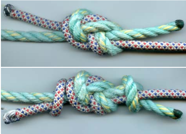
Fig. 7. A figure eight or Flemish bend (top, ABOK #1411) is generally secure with ropes of similar diameter, though various structures can arise from different threading and dressing methods. With careful dressing, some users report less jamming than multiple overhand bends (Fig. 8).
