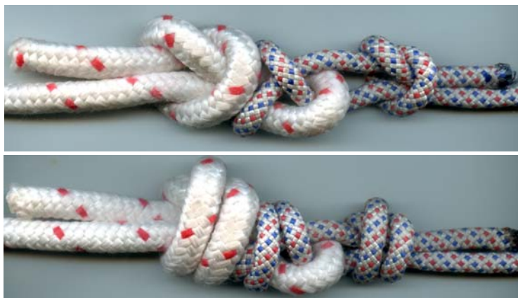
Fig. 6. The form of the secured sheet bend specified by NFPA for joining ropes of different sizes, but not for a human load (top).
